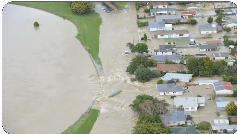
Image 6: Rangitāiki River stop bank breach, 06 April 2017 at 11.00hrs.
