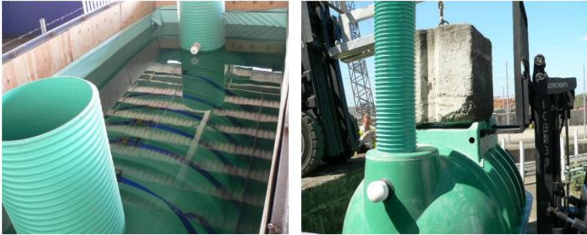
Figure 5-5. STEP tanks undergoing water tight and load testing (Source: Innoflow, 2017)
