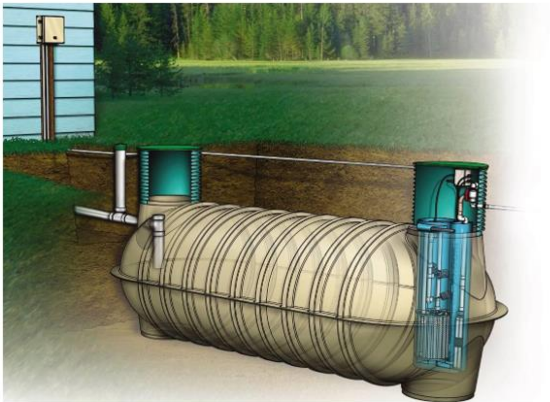
Figure 5-6. Schematic of Typical STEP Tank (Source: Innoflow, 2017)
